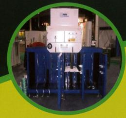
The twin (BP142) and triple (BP143) chambered balers offer versatility to clients looking to segregate and bale various material types.
